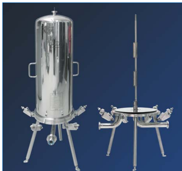
Figure 3: Pall's WSFZ lenticular housing provides flexibility in production. By installing internal center posts of different lengths, filtration can be run at 25, 50, 75 and 100% of capacity.
